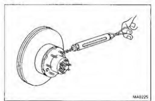
(g) Recheck the preload at the hub bolt.
